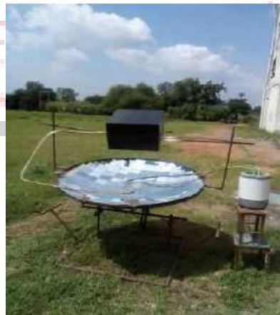
Figure 4 Previous experimental model of dish collector and receiver system.
