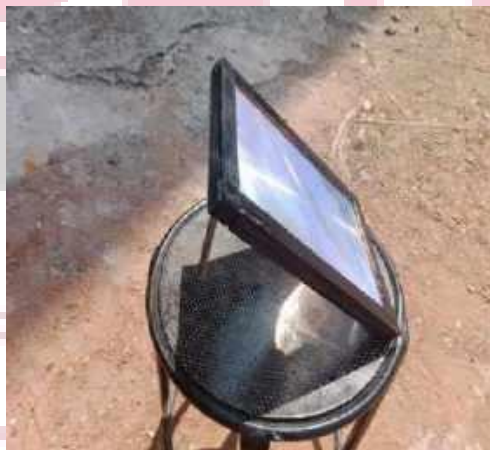
a) A rectangular Fresnel lens of glass
