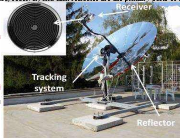
Figure 2 Parabolic dish collector system
